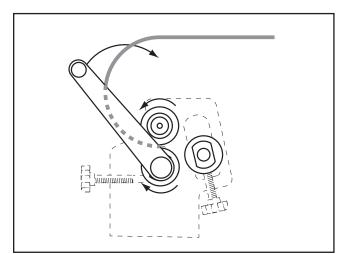
Figure 25. Re-inserting the workpiece.
